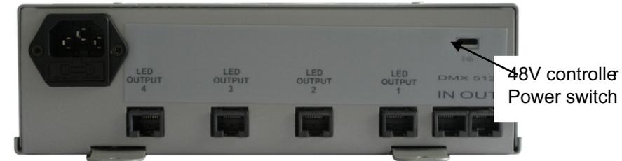
The DMX sockets (in and link through) allow control from a DMX desk or master-slave linking of units. Pin 1 is the leftmost pin in the above picture. The 48V switch puts out power on unused pins of the DMX sockets to power an external controller.
